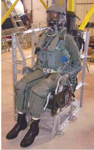
Figure 6. Large Case 6 Manikin in F-15 ACES II
