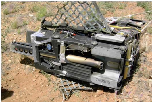
Figure 11. Test 1 Post Test Condition with CKU-5C/A
