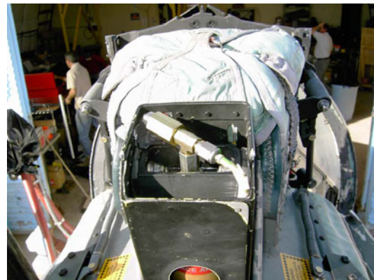
Figure 12. Catapult Pressure Cell and Tee Fitting
