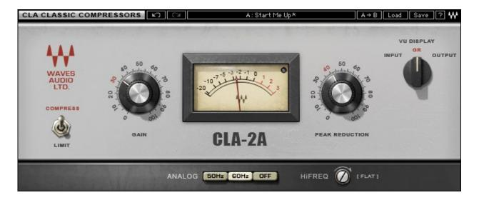
The CLA-2A offers 2 main controls for compression, as well as additional controls for fine-tuning.
