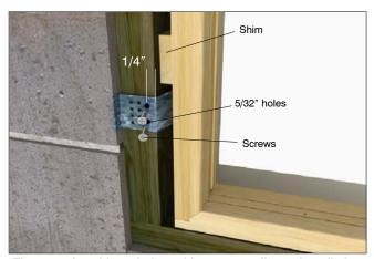
Figure 8: Attaching window with masonry clips or installation brackets.
