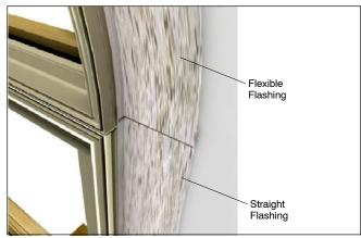
Figure 13: Use flexible flashing for radius head jambs
