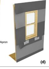
Figure 12: Sealing the Installation in building paper applications
