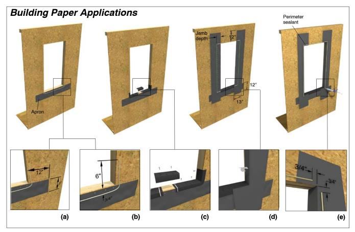
Figure 4: Rough Opening Preparation for construction methods using building paper and sill panning.
