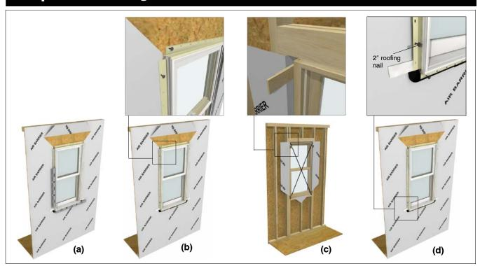
Figure 7: Positioning the window in the open-
