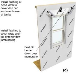
Figure 10: Sealing the Installation in air barrier applications
