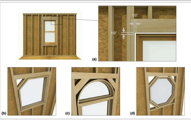
Figure 1: Typical rough and masonry openings.
