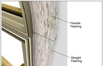
Figure 11: Use flexible flashing for radius head jambs
