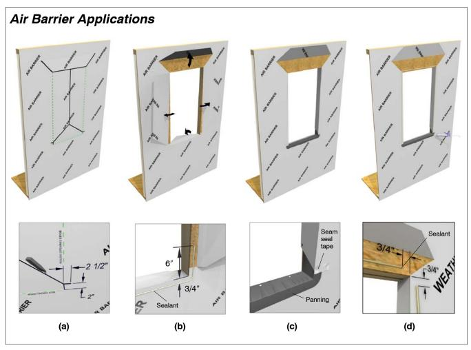
Figure 3: Rough Opening Preparation for construction methods using a continuous air barrier system and sill panning.
