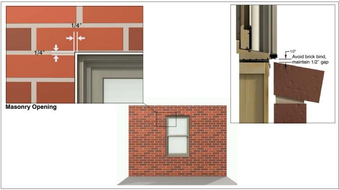
Figure 2: Typical rough and masonry openings.
