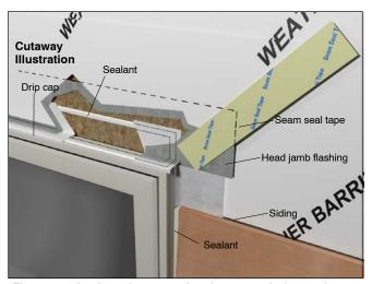
Figure 15: Apply perimeter sealant between window and exterior finish
