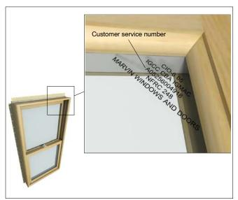
Figure 5: Etching on glass contains customer service number
