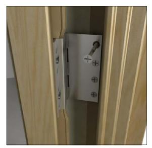
Figure 17: Install screw
