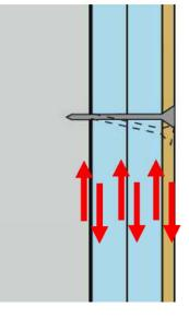
Shear and rotational resistance provided by fastener to wood connections
