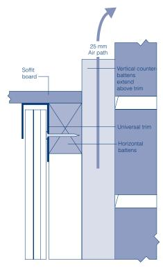
**Fig.40** Termination at soffit -Ventilated vertical cladding
