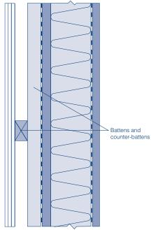
Fig.47 Vertical plankswith ventilation
