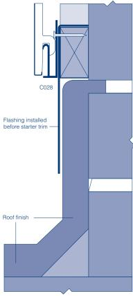
Fig. 7 Wall starter trim C028 above flat roof
