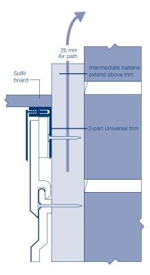
Fig.39 Termination at soffit -Ventilated horizontal cladding
