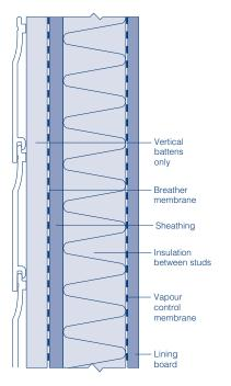
**Fig.46** Horizontal planks-without ventilation
