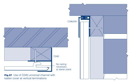
**Fig.28** Universal two-part trim C290/291 at head of cladding
