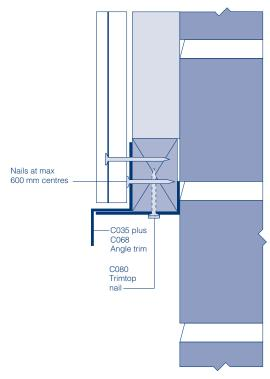
**Fig.25** C035 drip trim in conjunction with angle trim C068 to hide high level batten
