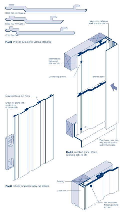
Fig.33 Finishing with a cut plank
