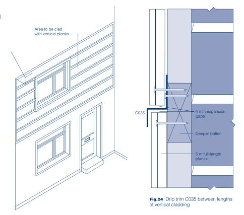
Fig. 23 Battening out
