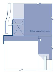
**Fig. 16** Drip trim C035 at window head with extended soffit board
