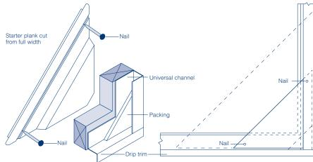
Front elevation Fig.34 Diagonal plank starter piece Isometric view Medicale lending them did had a defined position of ples in the second s 4 mm Alon Arma bah ards tot askarson Γwo-piece trims 4 mm Fig.35 Cutting intermediate planks to length -Packing Last plank fitted over preceeding and nailed through packing
