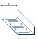
C061 (10 mm type) 30 x 15 mm Angle ventilator
