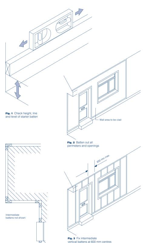
Fig. 4 Use two battens at internal and external corners
