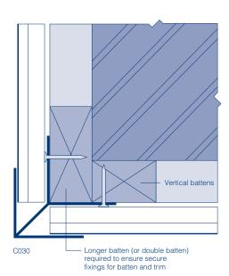
Fig. 12 Corner trim C030 at an external angle
