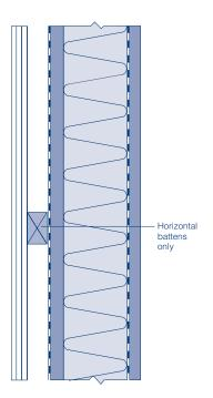
**Fig.48** Vertical planks-without ventilation
