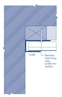
Fig. 10 Universal channel C026 at cladding reveal
