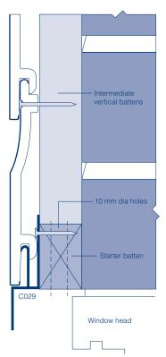
Fig. 6 Drip starter trim C029 at window head
