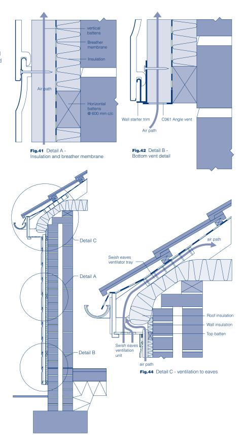
Fig.43 General view showing extent of insulation
