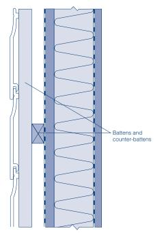
**Fig.45** Horizontal plankswith ventilation
