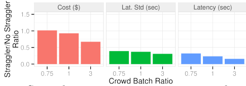
Figure 11: Straggler mitigation increases costs by 1 to 2 \times , improves latency by 2.5 – 5 \times , and variance by 4 – 14 \times .
