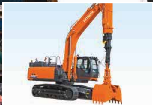
The telescopic arm extends and retracts smoothly with a full load.
