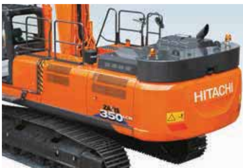
The detachable counterweight enhances the machine's versatility.
