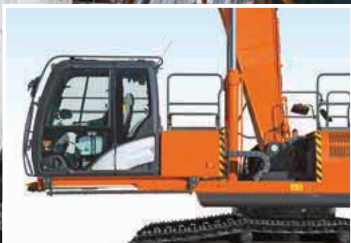
The sliding cab enhances visibility and safety.
