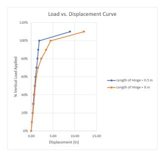
The load vs. displacement curve shows that the catastrophic failure now occurs at 100 kips compared to 140 kips in the previous loading condition.
