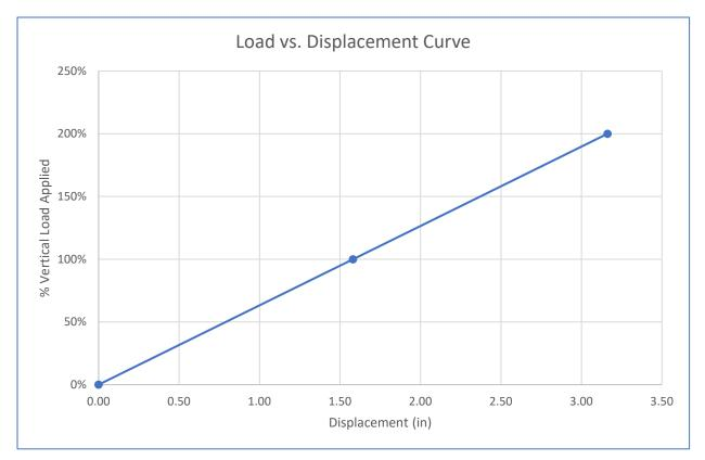
The vertical load vs displacement curve looks plotted using the above data shows a linear behavior.
