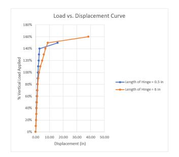
Let us now examine this same beam with an axial load applied in addition to the load applied at node #2. The load vs. displacement curve for this case is shown below.
