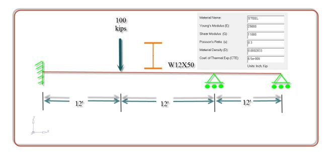
Looking at the results of this unit load, we see a 1.58" deflection at node 2, the point of load application.
