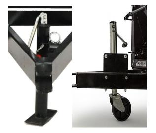
The swing away jack is used to hold the spreader in a safe level position when not connected to a tow vehicle. Use the jack to raise or lower the spreader for easy connection to the tow vehicle. With optional wheel attachment the spreader can be easily maneuvered around without having to attach the spreader to a tow vehicle. To rotate the jack remove the attached pin from the holder, rotate, and reinsert pin. To keep the jack from catching during use always raise the jack when in operation.
