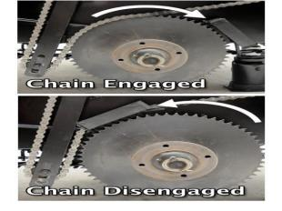
The operating lever labeled #2 in the above photo controls the chain engagement mechanism. This allows the chain to be disengaged and engaged one tooth at a time and helps keep the chain and sprocket in alignment. This also helps reduce unneeded repair, wear and tear, and breakage.
