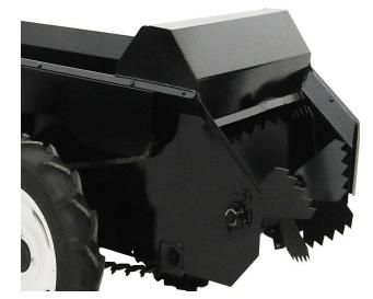
This exclusive feature offers two features. First is prevents any manure from flowing over the beaters, and second it acts as a shield for spray off. This helps with "clean" spreading and prevents spray off from hitting the operator.
