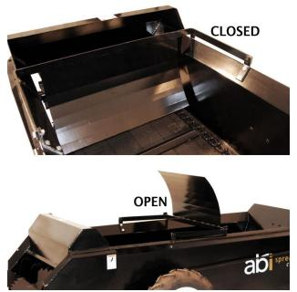
The optional end gate is used to prevent manure from spilling out during filling or transportation, and to help further deflect material from the operator during spreading. The end gate should never be down when spreader is in use. For models 25 - 50the end gate must be operated manually. For larger models 85 - 130 there is an optional hydraulic lift arm. Having this down during use may cause damage to the hood or tool.
