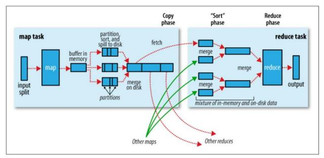
Figure 6-6. Shuffle and sort in MapReduce
