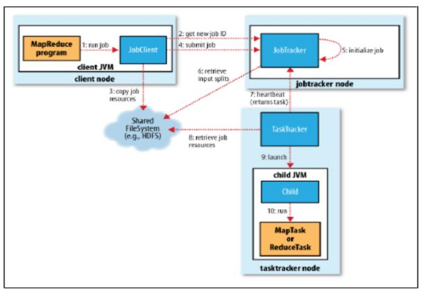
Figure 6-1. How Hadoop runs a MapReduce job using the classic framework
