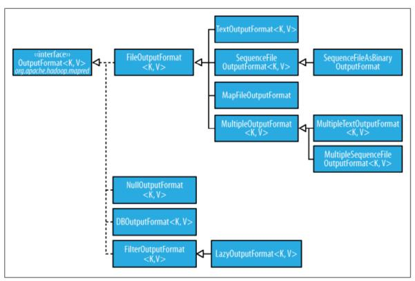
*Figure 7-4. OutputFormat class hierarchy*
