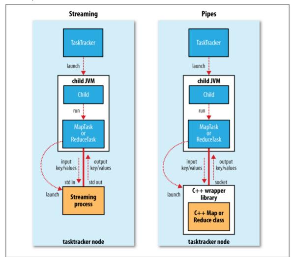
Figure 6-2. The relationship of the Streaming and Pipes executable to the tasktracker and its child
