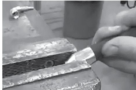
(The internal barbs are LH thread.)
