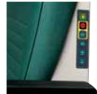
Backlit flat overlay switches are easy to see in a darkened room.
