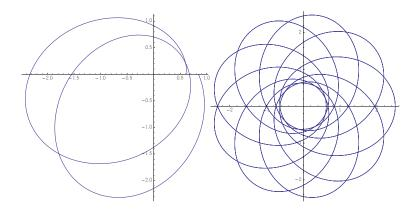
Figure 3.4: Orbit of a fictitious gravitational potential with additional  $\frac{1}{r^2}$  contribution to the potential. Note, orbits are no longer closed. The left panel shows the path after two orbits, the right panel after 20 orbits. We used  $\epsilon = 0.6$  and  $\alpha = 0.9$ .
