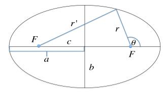
Figure 3.1: Ellipse with semi-major axis a and and semi-minor axis b. F and F' are the foci of the ellipse, c the distance between the center and the foci.
