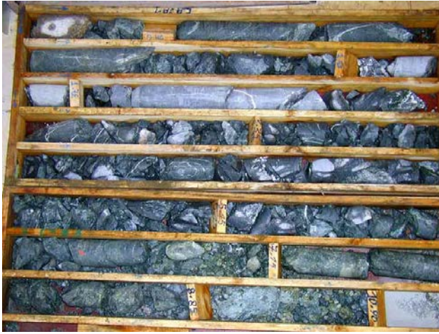
Figure 45: Drill cores from a weakness zone. It is very difficult to assess the outlook/characteristics of the zone from such information.
