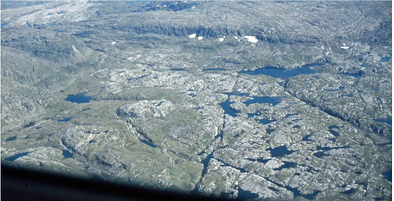
Figure 5: Aerial view of a glacier eroded terrain surface without vegetation and loose materials. Important geological features can be observed as lines, indicating weakness (fault) zones. Also, distribution of old Precambrian rocks and Cambrian – Silurian rocks can be assessed a different (greenish) colour. In addition, the pattern of joints can be seen.
