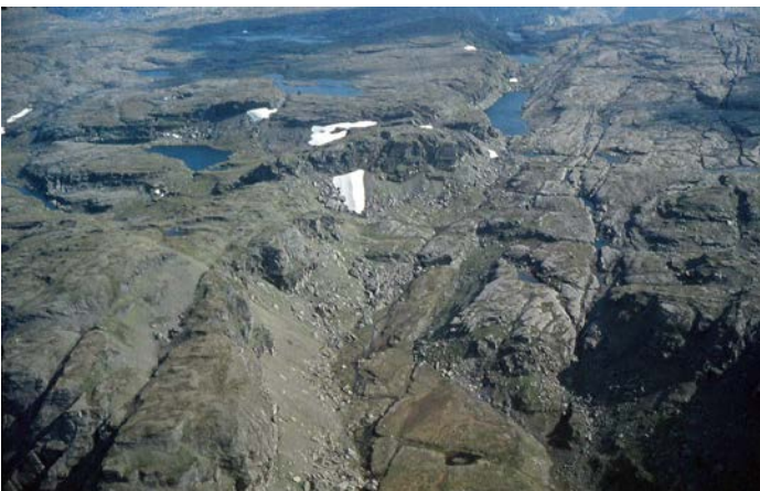
Figure 38: Interpretation of aerial photos of exposed, almost fresh rocks gives valuable information rockmass conditions. Combined with field observations, good assessments can be made of the conditions in the planned tunnel or cavern.
