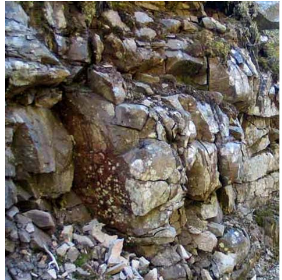
Figure 41: Irregular jointing. Block sizes varying from 1 dm 3 to 100 dm 3 . What block size (or RQD) to be applied?
