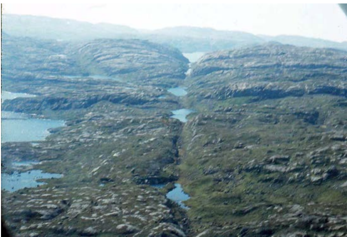
Figure 3: Large weakness zones (fault zones) can easily be detected in the terrain surface as depressions.
