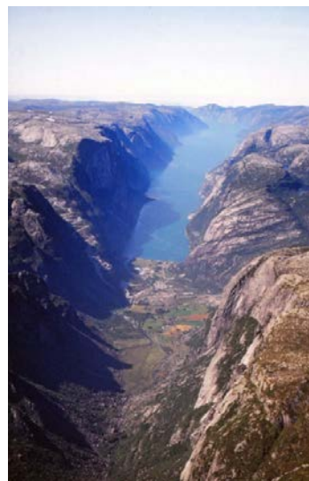
Figure 3: Large weakness zones (fault zones) can easily be detected in the terrain surface as depressions.
