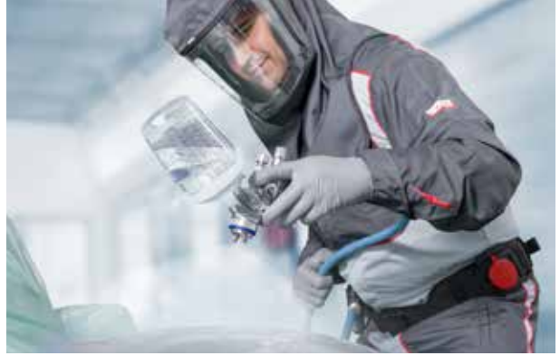
Optimum personal breathing protection with clean compressed air supplied by e.g. the SATA filter 484 with activated charcoal filter stage.
