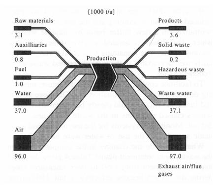
Figure 10: Overview of the materials flows in the textile mill (including raw and auxiliary materials, water and air)
