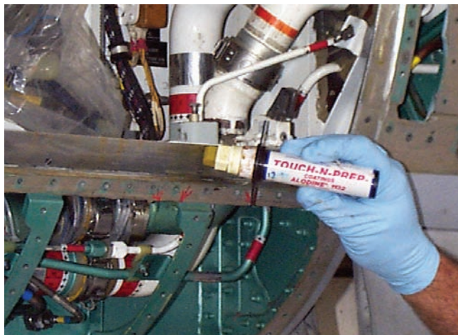
Figure 5-3. Application of TNP Pen on Aluminum Substrate
