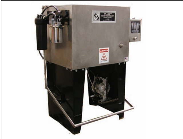
Figure A-6. Paint Gun Washer
