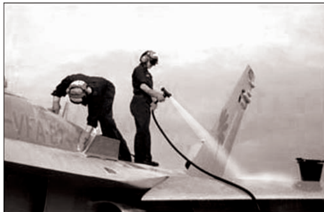
Figure 2-3. Washing and Rinsing of Aircraft Surfaces
