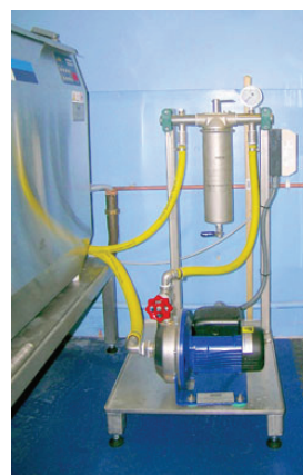
Si-80 wash stage with 10" filter and two stage cascade rinse with P2S size closed loop filtration, active carbon filter and deioniser.
