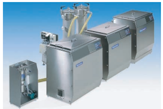
Si-80 wash stage with 10" filter and two stage cascade rinse with P2S size closed loop filtration, active carbon filter and deioniser.
