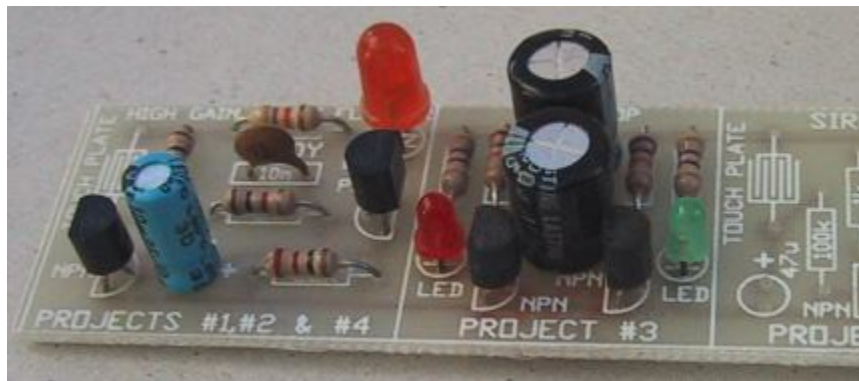
The Flip Flop components added to the board
