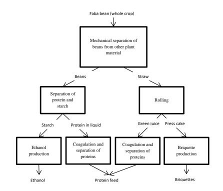
Figure 8. The green crop biorefinery considered in Paper III (Figure from Paper III).
