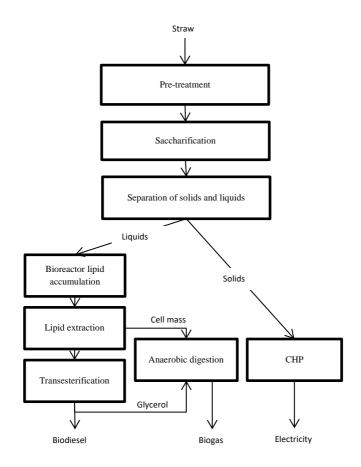
Figure 7. The biorefinery system considered in Papers IV and V.
