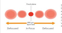
Single SLT aiming beam focusing is easily achievable at focal plane, producing crystal clear spot with visible internal inner rings.
