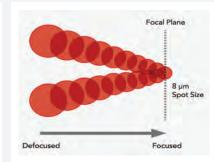
YAG twin aiming focusing system allows both beams to converge together at the focal target to create a sharp and precise spot.
