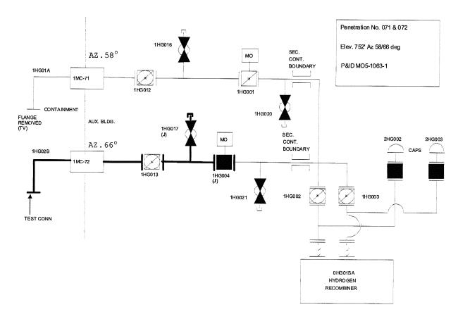
Filled in valves = shut Test Volume in Bold Test Valves: (1HG017 & 1HG004)
