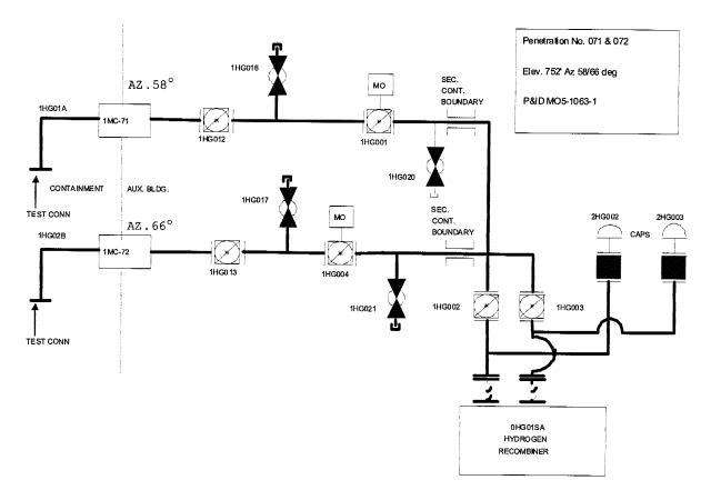
Filled in valves = shut Test Volume in Bold Test: (Closed Loop)
