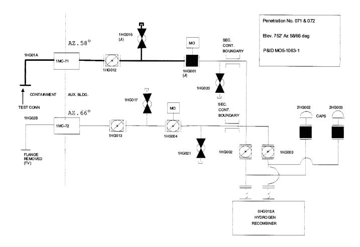
Filled in valves = shut Test Volume in Bold Test Valves: (1HG016 & 1HG001)
