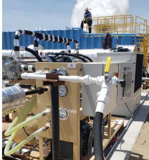
Figure 18: Supercritical CO 2 Injected Into the Well Just After Opening
