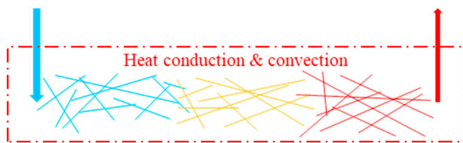
Fig. 1. Schematic diagram of the heat transfer mechanism in conventional geothermal energy recovery with a pair of vertical wells. Colours represent working fluid temperatures ranging from cold (blue) to hot (red).
