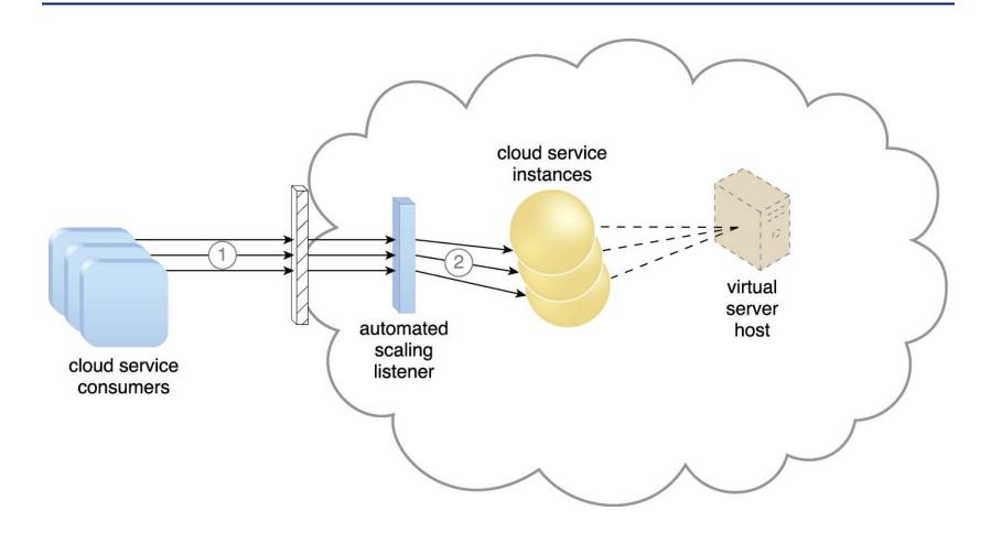
Cloud service consumers are sending requests to a cloud service (1). The automated scaling listener monitors the cloud service to determine if predefined capacity thresholds are being exceeded (2).
