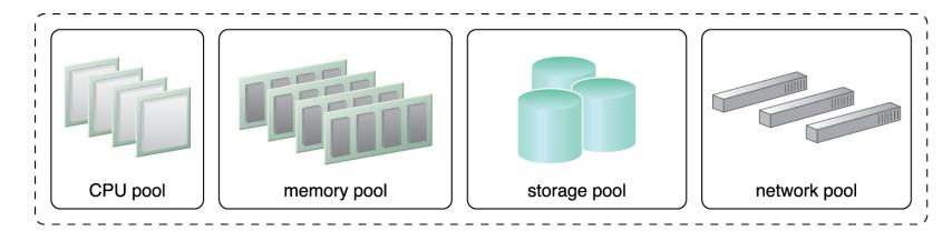
A sample resource pool that is comprised of four sub-pools of CPUs, memory, cloud storage devices, and virtual network devices.
