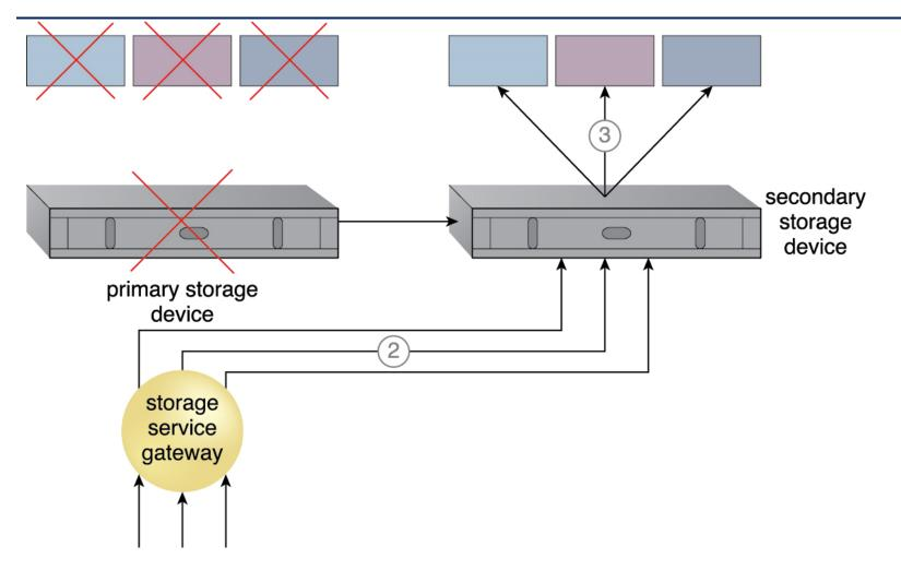
The primary storage becomes unavailable and the storage service gateway forwards the cloud consumer requests to the secondary storage device (2). The secondary storage device forwards the requests to the LUNs, allowing cloud consumers to continue to access their data (3).
