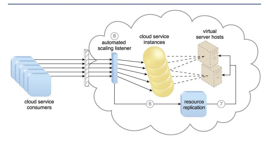
The automated scaling listener sends a signal to the resource replication mechanism (6), which creates more instances of the cloud service (7). Now that the increased workload has been accommodated, the automated scaling listener resumes monitoring and detracting and adding IT resources, as required (8).
