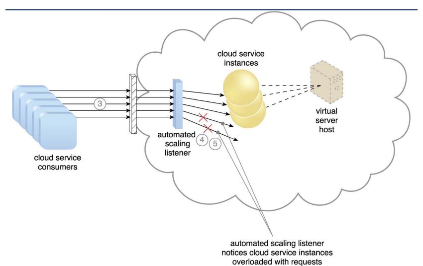
The number of requests coming from cloud service consumers increases (3). The workload exceeds the performance thresholds. The automated scaling listener determines the next course of action based on a predefined scaling policy (4). If the cloud service implementation is deemed eligible for additional scaling, <sup>11</sup> the automated scaling listener initiates the scaling process (5).
