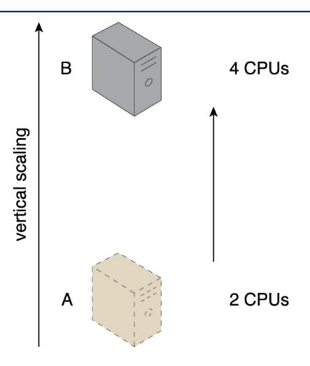
An IT resource (a virtual server with two CPUs) is scaled up by replacing it with a more powerful IT resource with increased capacity for data storage (a physical server with four CPUs).
