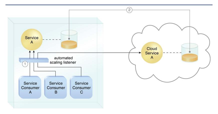
An automated scaling listener monitors the usage of on-premise Service A, and redirects Service Consumer C's request to Service A's redundant implementation in the cloud (Cloud Service A) once Service A's usage threshold has been exceeded (1).
