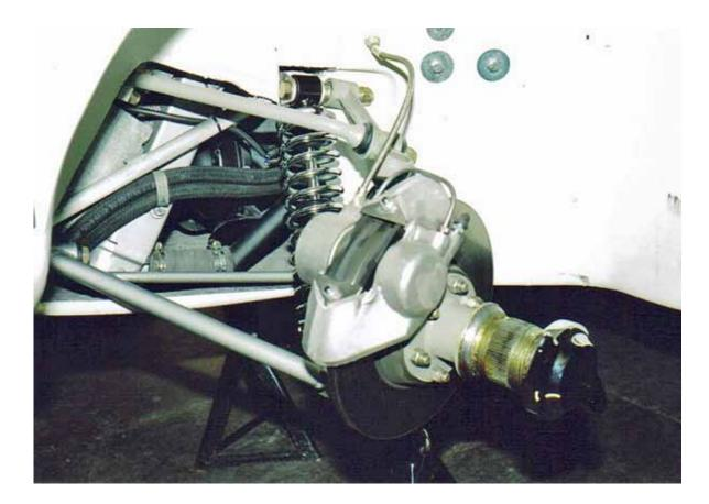
Any safety-critical parts not replaced were carefully inspected, crack-checked and refinished. The steering column rubber joint was replaced with a needle-roller u-joint assembly and the rack carefully rebuilt. Incorrect steering arms on this car were replaced with Standard items, bent to the correct angle just as probably done at Lotus. Cast-iron front calipers were replaced with alloy ARs. Shim
