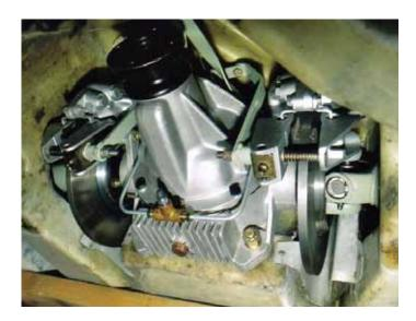
NR calipers were on the wish list but aside from the need to change to a Series 1 diff case and handbrake, it was decided that being sprung mass the smaller performance gain would not be worth the expense. Stuart desired weight savings wherever possible. In the end we only left out the cabin insulation, carpet and miscellaneous trim.
