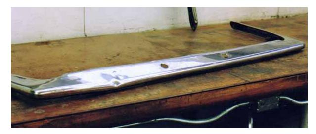
I have not been able to find a reliable metal finisher who is patient enough to massage these delicate hand-made pieces back into shape, so I have spent many hours learning and practicing. The flat expanse on the rear bumper is especially challenging since the slightest distortion is plainly visible. With great patience and various steel dollies, wood blocks, rubber mallets, files and felt marking pens the
