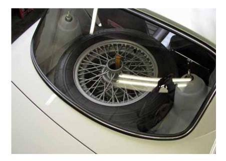
We installed a plastic rear window, but added safety equipment and more fuel. I argued against deleting the heater & ducts, reasoning that effective defogging might be a greater advantage than a pound or two less mass. An aluminum radiator was tempting, but the desire for originality outweighed.
