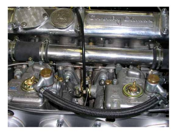
The original throttle pedal for SUs needed its lever extended to obtain enough cable stroke at the carb levers. A hairpin return spring like the one on Elan Webers was made from piano wire.
