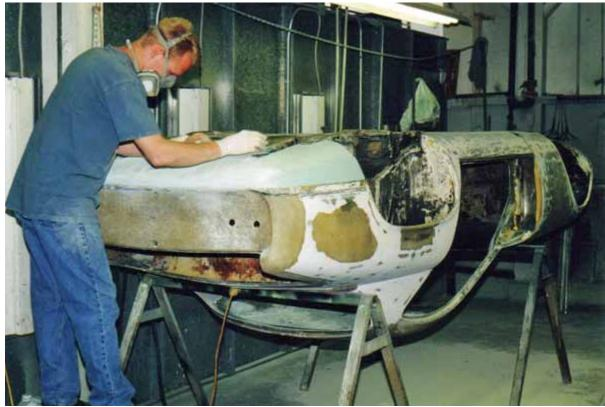
White is good original primer/surfacer. Dark patches are gel-coat repairs with glassfiber veil. Original gel-coat is not colored.
