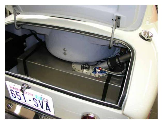
We built an FIA-spec fuel cell to look like the Le Mans tank. The fitted foam-filled bladder holds about 32 liters (8 ½ gallons).
