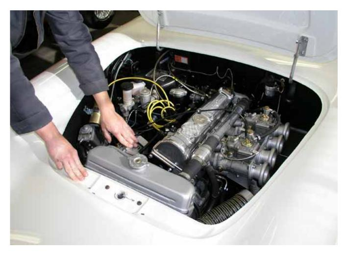
Though we planned to duct intake air to the carbs I did an initial road test without a duct and found engine bay temperature at the intakes was rarely below 40 deg C and climbed past 60 deg C when stopped and idling in 20 deg C ambient. With the addition of a 3-inch duct from in front of the radiator to the trumpets temperature rarely rose beyond 40 deg C, and declined quickly to near ambient at speed.
