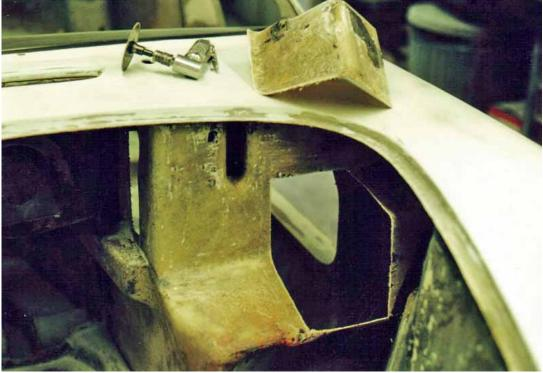
Footwell section carefully marked, then cut out with Rem-Grit cutting disk.
