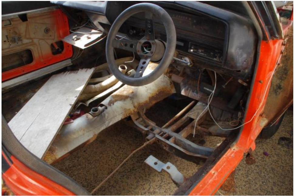
Tim has cut out the rusty floors. The new ones are waiting in the tray of the ute (below) The uppers bits of the car are not bad.
