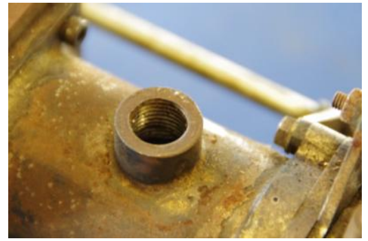
This engine was meant to be water cooled. Here is the upper connection to the water jacket.
