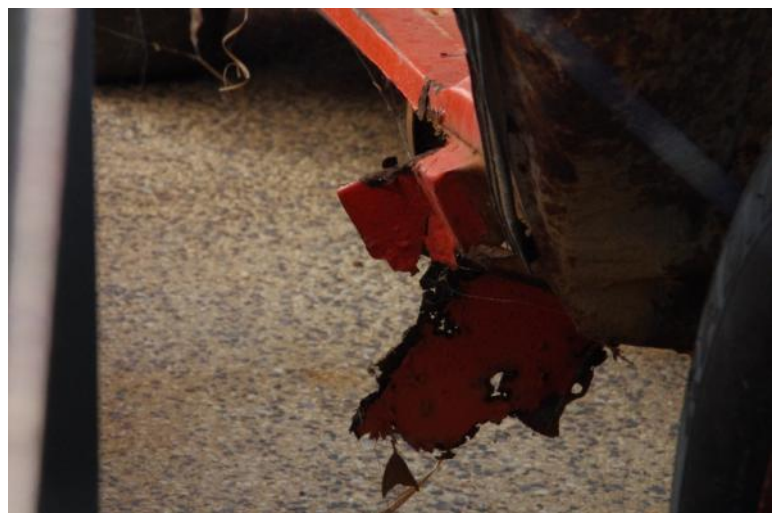
Below: The sills are a bit poor.
