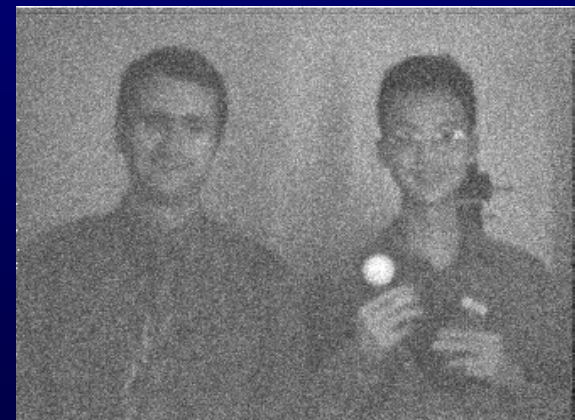
1000x less light: 200 millilux, 60 Hz, F/1.4
