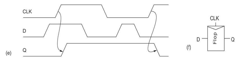
**FIG 1.31** CMOS positive-edge-triggered D flip-flop
