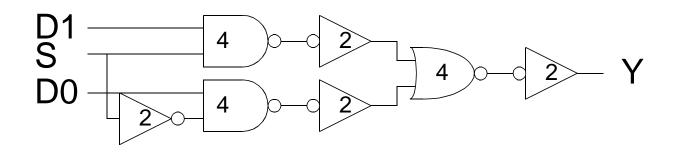
How many transistors are needed? Too Many !!! (20 transistors)
