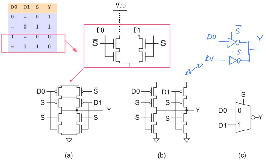
FIG 1.28 Inverting multiplexer
