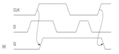
FIG 1.31 CMOS positive-edge-triggered D flip-flop
