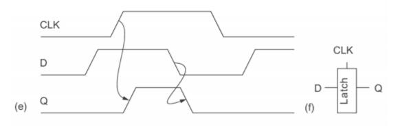
FIG 1.30 CMOS positive-level-sensitive D latch
