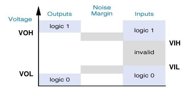
Figure 1-2 Logic values and noise margins.
