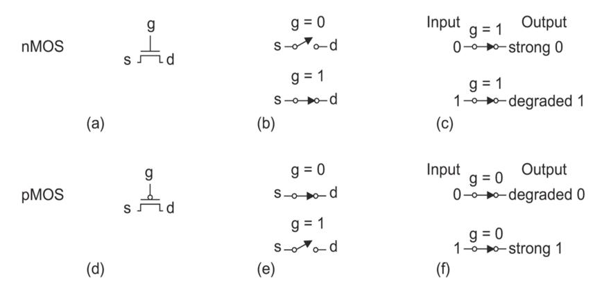
**FIG 1.19** Pass transistor strong and degraded outputs
