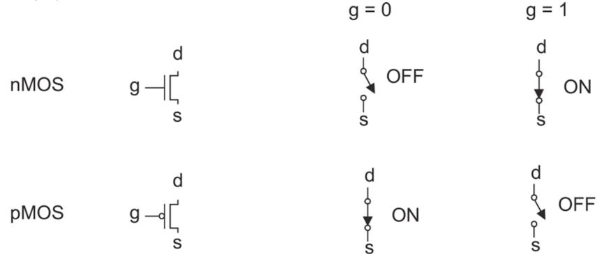
**FIG 1.9** Transistor symbols and switch-level models
