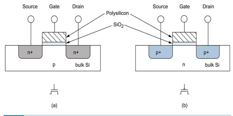
FIG 1.8 nMOS transistor (a) and pMOS transistor (b)
