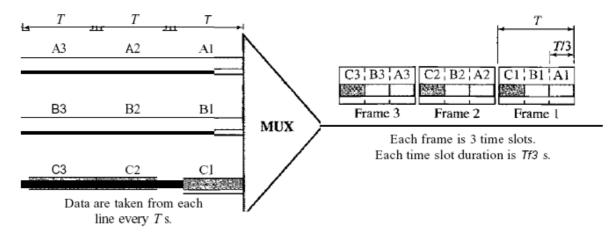
Figure 7 Synchronous time-division multiplexing
