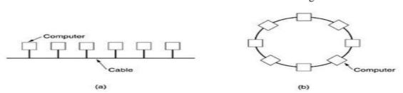
Fig.1: Two broadcast networks . (a) Bus. (b) Ring.
