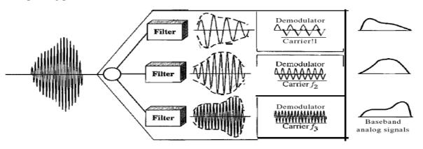
Figure 3 FDM de-multiplexing example
