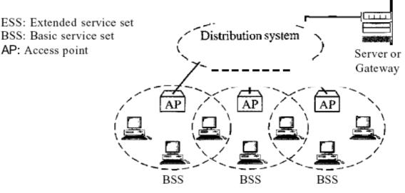
Figure 10 Extended service sets (ESSs)
