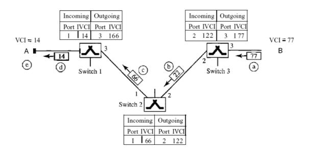
Figure 5 Setup acknowledgments in a virtual-circuit network
