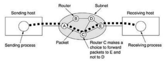
Fig.3.1: A stream of packets from sender to receiver.
