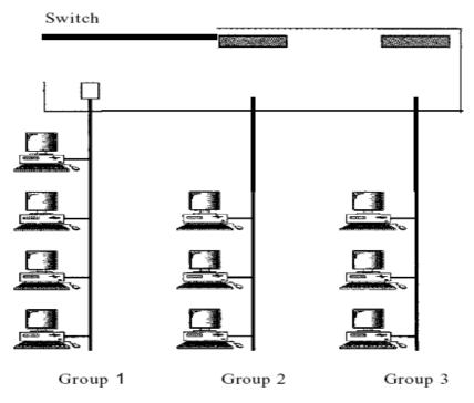
Figure 6 A switch connecting three LANs
