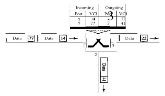
Figure 2 Switch and tables in a virtual-circuit network
