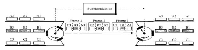
Figure 8 Interleaving
