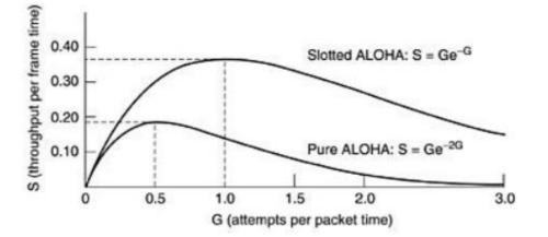
Fig.3 Throughput versus offered traffic for ALOHA systems.
