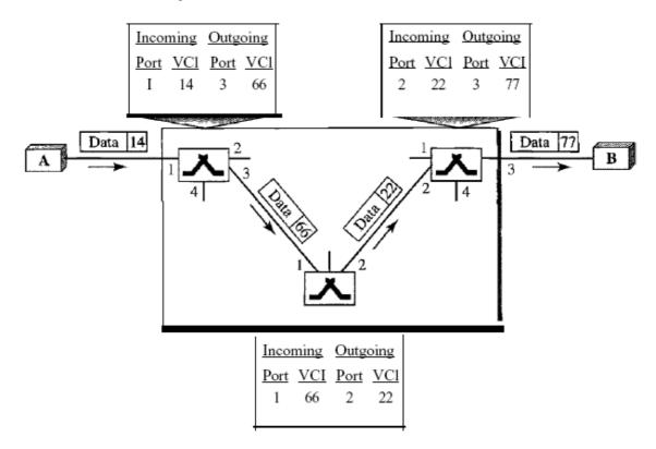
Figure 3 Source-to-destination data transfer in a virtual-circuit network
