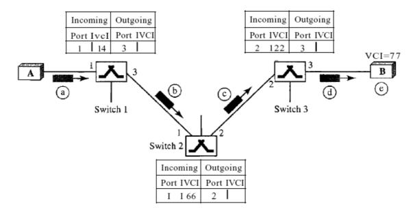
Figure 4 Setup request in a virtual-circuit network
