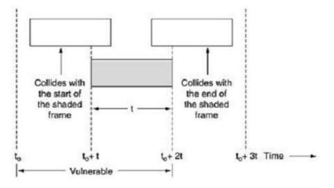
Fig.2. Vulnerable period for the shaded frame
