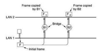
Fig.3. Two parallel transparent bridges.
