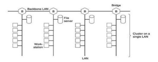
Fig.1 Multiple LANs connected by a backbone to handle a total load higher than the capacity of a single LAN.
