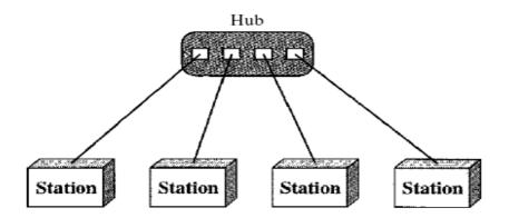
One big disadvantage of a star topology is the dependency of the whole topology on one single point, the hub. If the hub goes down, the whole system is dead. Although a star requires far less cable than a mesh, each node must be linked to a central hub. For this reason, often more cabling is required in a star than in some other topologies (such as ring or bus).
