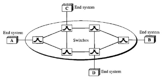
Fig a: Virtual-circuit network
