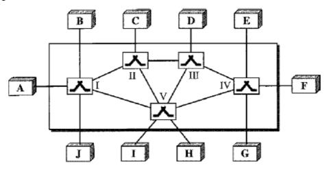
The end systems (communicating devices) are labeled A, B, C, D, and so on, and the switches are labeled I, II, III, IV, and V. Each switch is connected to multiple links.
