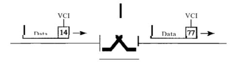
Figure 1 Virtual-circuit identifier
