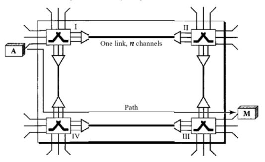
Fig: A trivial circuit-switched network
