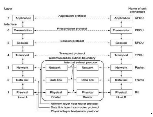
Fig.4: The OSI reference model
