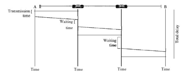
Fig: Delay in a datagram network
