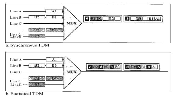
Figure a TDM slot comparison
