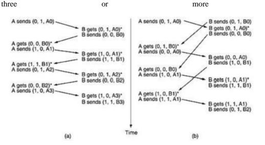
Fig.9.2 Two scenarios for protocol 4 (a) Normal case (b) Abnormal case. The notation is (seq, ack, packet number). An asterisk indicates where a network layer accepts a packet.
