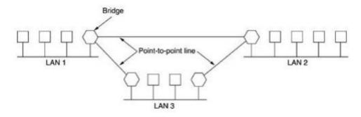
Fig.5. Remote bridges can be used to interconnect distant LANs.
