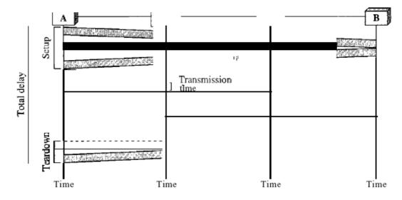
Fig: Delay in a virtual-circuit network
