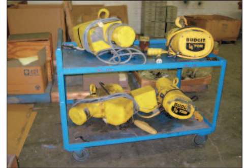
View of Budgit Chain Hoists
