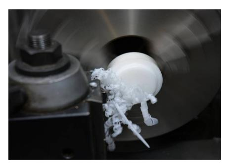
This involved some lathe turning and milling. The milling required accurate indexing for drilling holes for the balls, this could have been done by writing some simple G code to use CNC features but I thought it both quicker and better for the purposes of demonstration to use a rotary table with chuck. The lathe work could also be done on the mill with the rotary table if a lathe is not available.
