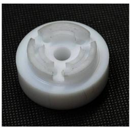
Firstly a spigot was turned to fit inside the aluminium outer tube, then the ball holes were made using a flat ended 6.35 mm (1/4") milling cutter. The holes were accurately made to the same depth and the flat bottom was used to ensure a good vertical location of the balls. A separate test had shown that making a hole with the milling cutter gave a very slight interference fit on the balls which enabled their fitting without glue.
