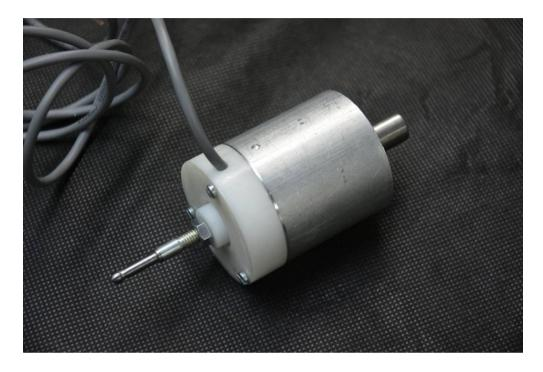
The main body was drilled 2.5 mm and tapped for the M3 screws.
