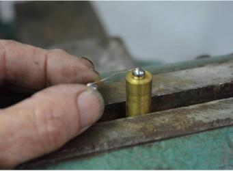
I used very thin copper wire for the connections because it was easier to solder to the balls. The balls were supported in a brass rod with a hole to sit in. The bar was first warmed as a heat source to keep the balls warm to facilitate the soldering. A small drop of non-rosin based flux was put onto the flat section and a touch with a soldering iron quickly tinned the ball ready to take the pre-tinned copper wire.
