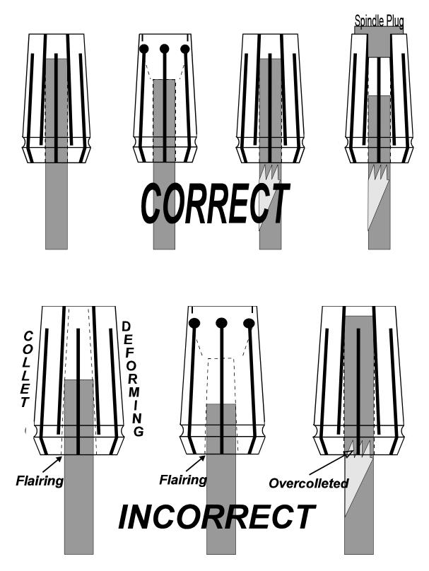
Heat is the biggest enemy of the tool, and the first place the heat goes from the tool is into the collet. It is also important to note that collets are made of spring steel that can, and will over a period of time lose it's elasticity and harden, making it increasingly tougher to tighten adequately. As this hardening takes place, the steel does not fatigue evenly and often causes the collet to grip tighter on one side than the other, creating runout in the tool.
