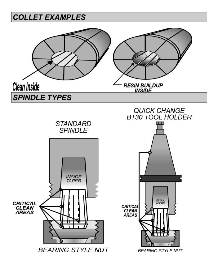
As is the case with collet types, there are two spindle nut types as well. Both types are not always available depending on the spindle type itself.
