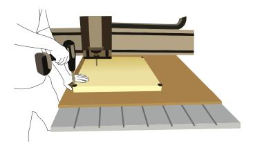
**PRE-DRILL HOLE5** in your material either on a work bench or off the side of the machine.
