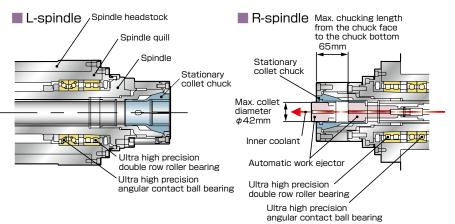
L-spindle Power Diagram
