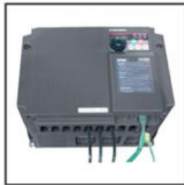
Spindle Control with VFD
