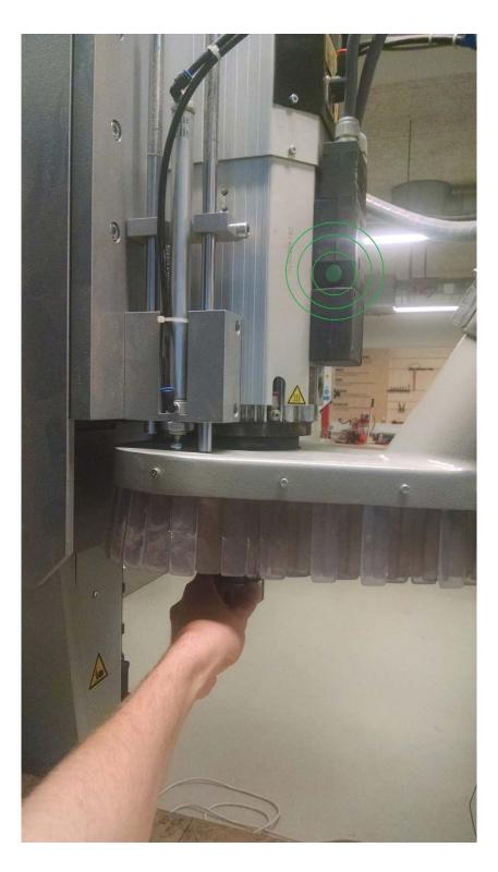
You can manually load and unload tools into the machine.
