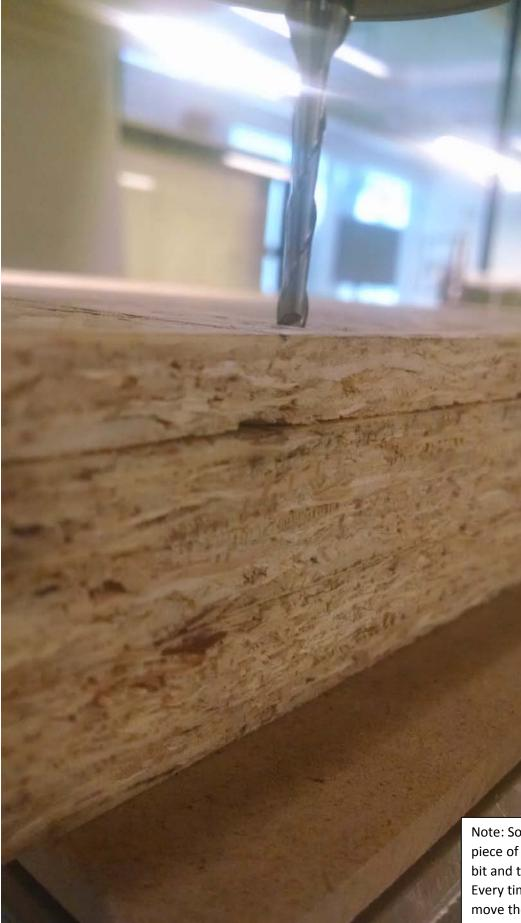
This is really close to the zero point, but it's not fully touching. I got to this point while holding the "Slow" button, so now I'm going to release the button and tap the Z- key a few times until the bit is just touching the surface.
