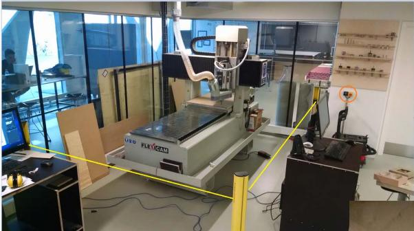
This switch resets the barrier. Turn it back and forth – once in the clockwise position, once counter-clockwise – to activate the barrier. The light barrier warning in the HMI will disappear once the barrier is active.
