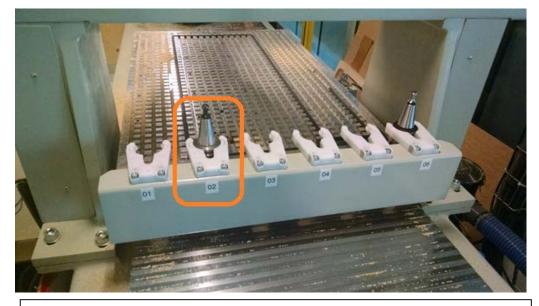
Check for error messages before running this command– the light barrier might be broken, for example – the machine needs all error messages clear before it will tool change. So now we have a smaller bit in the tool head.
