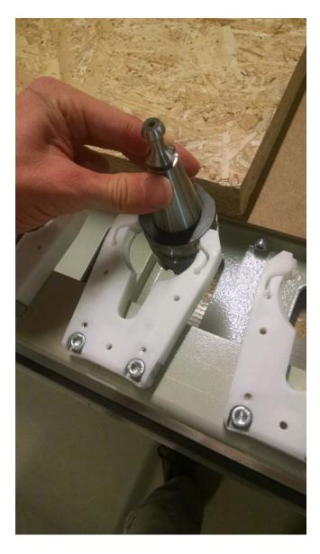
When you're putting a new tool in the rack, make sure the machine isn't holding a tool that belongs in that spot.
