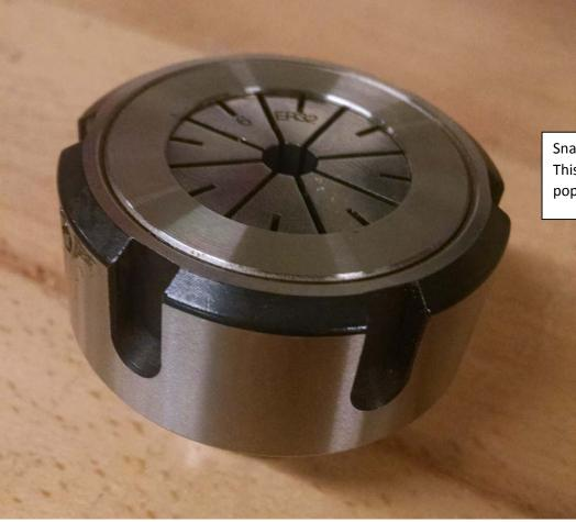
Snap on a round chuck onto the top. This should fit over the top and pops in place...
