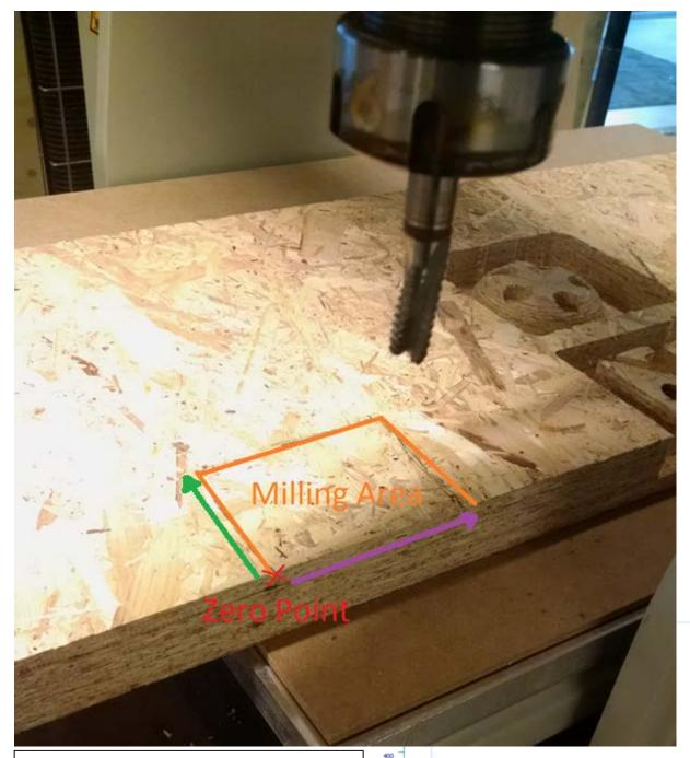
Our file's zero point is the bottom left of the shape. Let's set our zero point right on the material's corner to save room.
