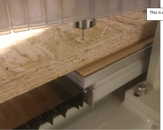
Note: The vacuum pump needs to be on when you're setting your zero point; you don't want your material moving at all after the point is set!
