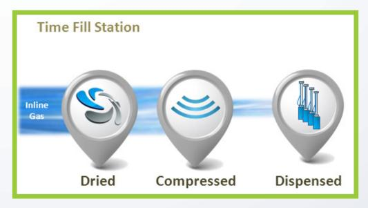
Fleets of vehicles that return to central locations for periods of time frequently utilize the time-fill configuration. This is a lower cost option and is a preferred method of refueling refuse trucks, school buses and other fleets with similar refueling requirements. Time-fill stations have significantly lower equipment and installation costs because they do not require storage, priority, or sequential refueling components.
