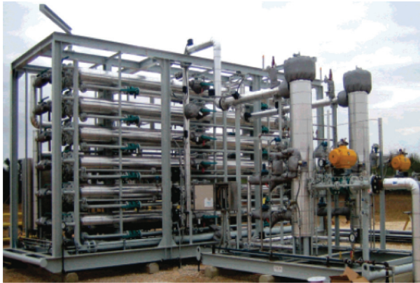
(b) Cellulose acetate membrane plant, which uses the spiral-wound configuration for the removal of CO 2 from natural gas (Baker and Lokhandwala 2008, page 5).
