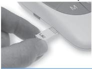
Slide the new code chip into the code chip slot until it snaps into place.
