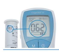
Confirm that the number displayed matches the number on the test strip container, then press the M button ...
