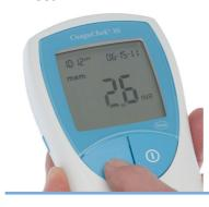
The most recent test result appears. The letters **mem** indicate that you are viewing a result in memory. The time and date of the test also appear.
