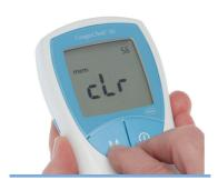
With the meter turned off, press and hold down the M button . While you are holding down the M button, press the ON-OFF button and then hold down both buttons for at least 5 seconds.
