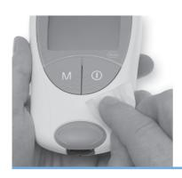
Remove the lancet from the lancet device. Place the used test strip and lancet in a punctureproof container with a lid. Turn the meter off .
