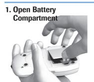
With the meter turned off, turn it over. Press the latch gently inward and lift the cover. Remove the old batteries, if necessary.
