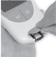
With the meter turned off, use your thumbnail to open the cover of the test strip guide by pressing its front edge upward.
