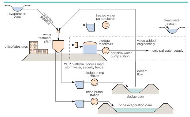
Figure 15 Water reclamation project at the Optimum mine, South Africa – schematic diagram showing the raw water collection, treatment, storage, distribution and sludge and brine disposal (Cogho, 2012)
