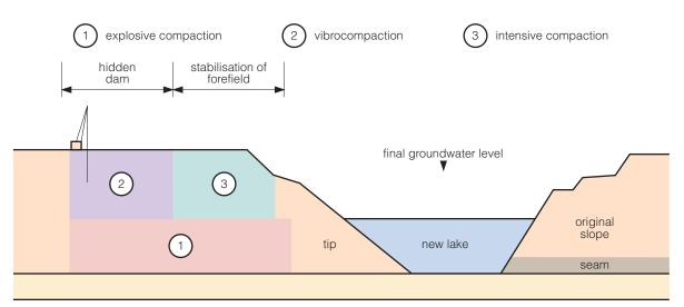
Figure 21 Combination of methods for compaction (Kuyumcu, 2011)
