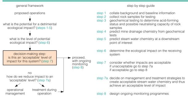
Figure 9 General framework and detailed step-by-step guide for predicting and managing water quality impacts from mining on streams (Cavanagh and others, 2010)
