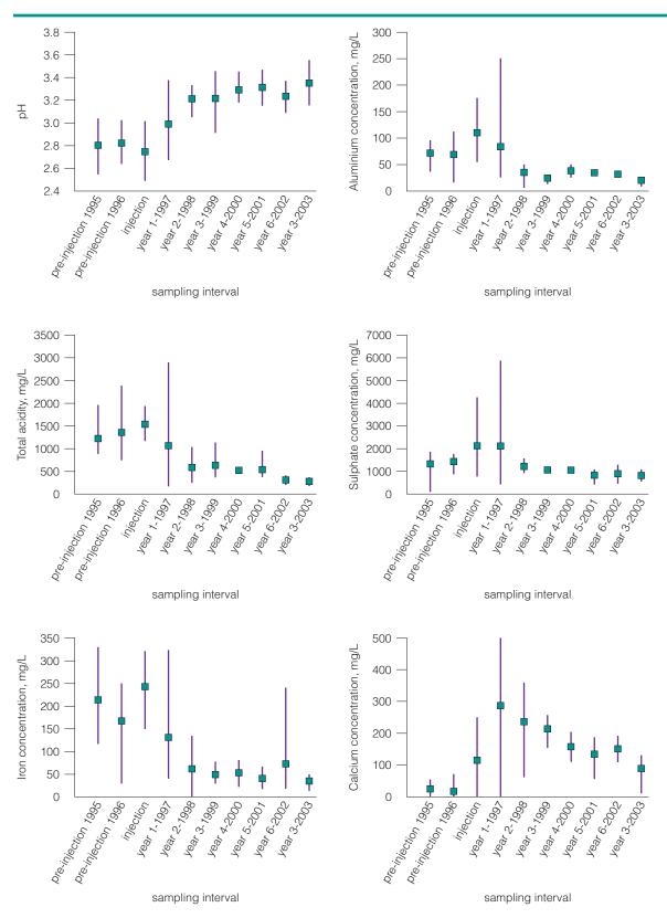
Figure 14 Concentrations of various acid mine drainage parameters before and after placement of the grout (Bulusu and others, 2005)
