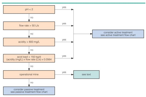
Figure 12 Flow chart to guide selection between active and passive treatment for AMD (Cavanagh and others, 2010)
