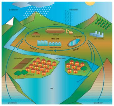
Figure 8 Flows of water to and from a mine site (ICMM, 2012a)
