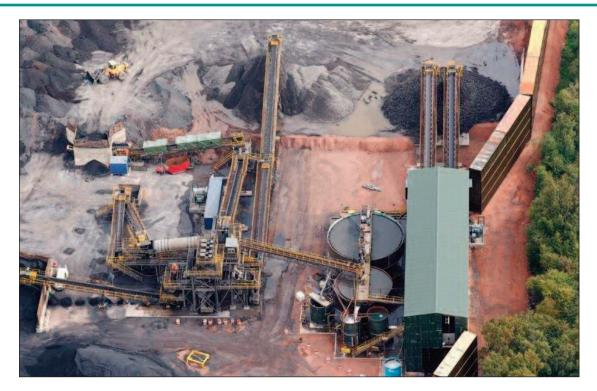
Figure 26 Former Langton Colliery Spoil Heap Coal Recovery and Reclamation Scheme (Photograph courtesy of RecyCoal, 2012)
