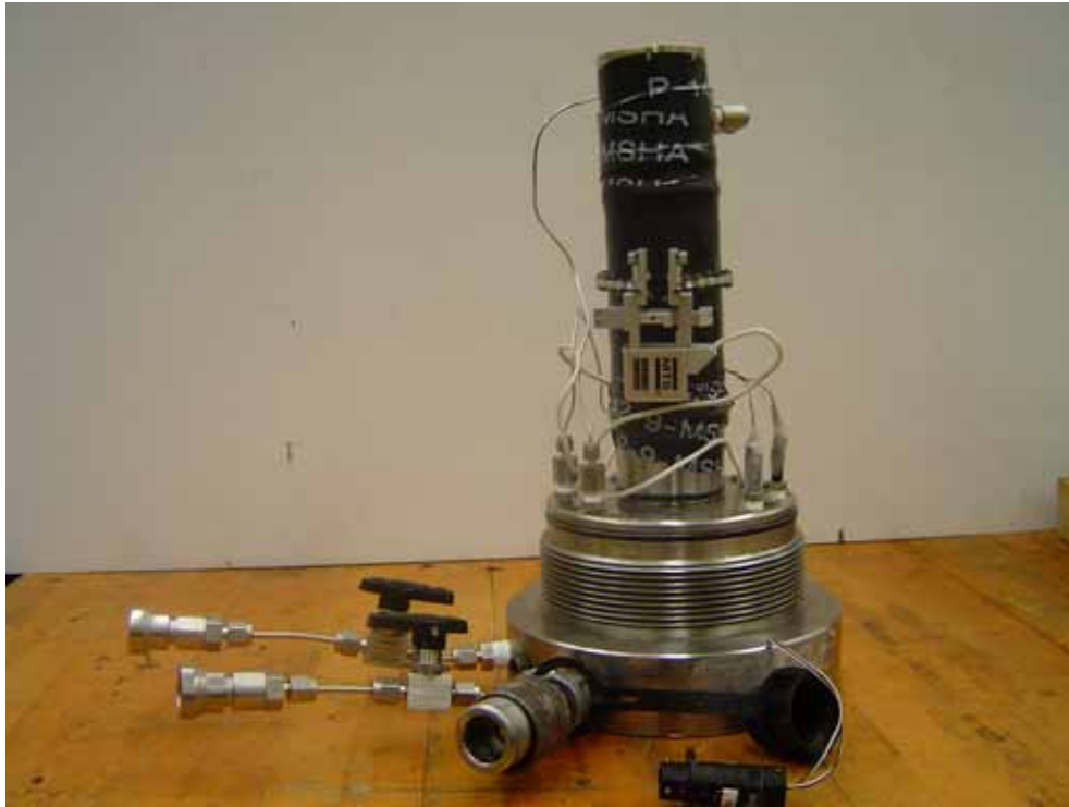
Figure 1: Triaxial cell base along with perforated steel disks, core and circumferential extensometer.
