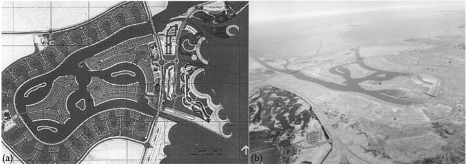
Figure 9.11 Doha West Bay Lagoon using artificial headlands (a) concept plan; (b) post-construction.
