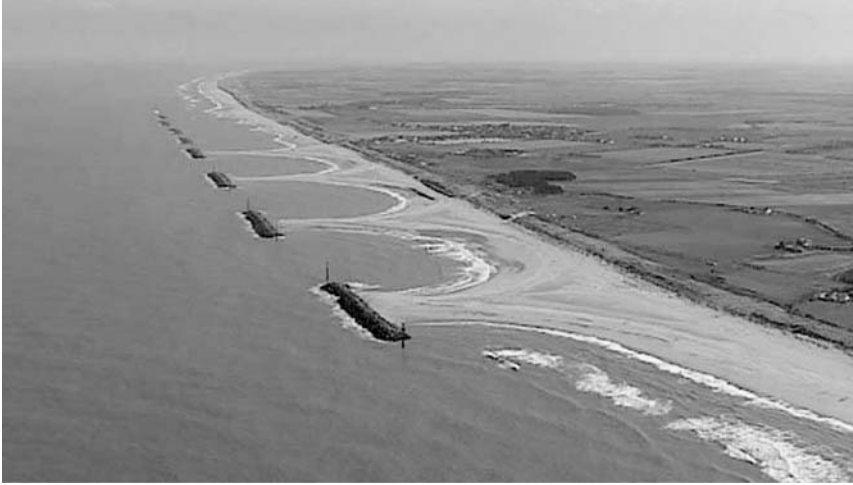
Figure 1.8 Tombolo formation, Happisburgh to Winterton Coastal Defences (reproduced by kind permission of Halcrow).
