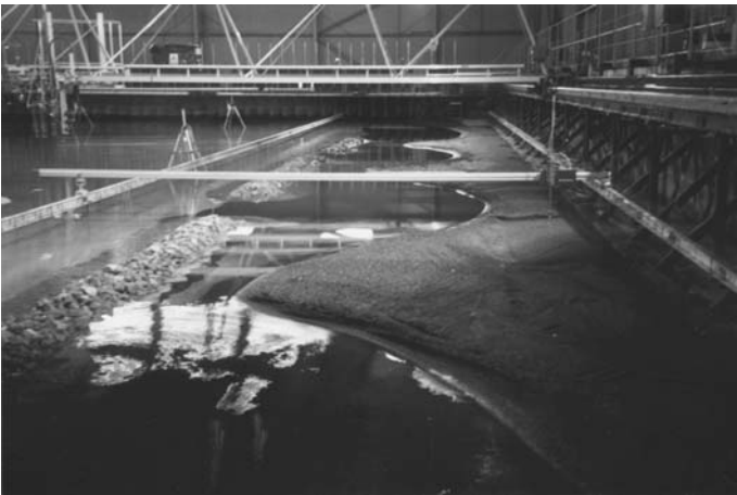
Figure 8.2(b) Mobile bed anthracite model.
