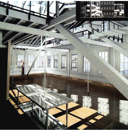
Intumescent coatings applied to wood structural elements in an historic manufacturing building converted into residential condominiums.
