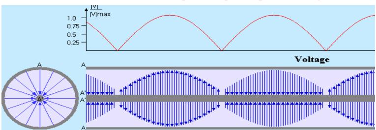
Voltage on coaxial line depends on time and position. The VSWR=indefinitely large.
