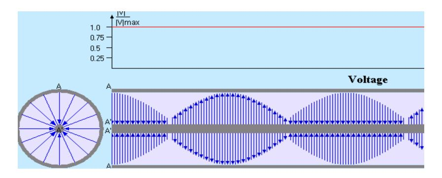
Voltage on coaxial line does not depend on time and position, because the load is matched.
