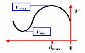
For an inductive reactance, a voltage maximum is closest to the load and
