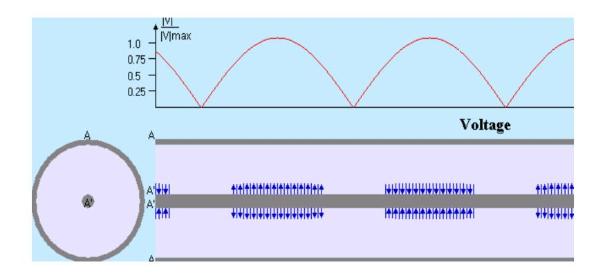
Voltage on coaxial line depends on time and position, and at nodes, goes to zero .
