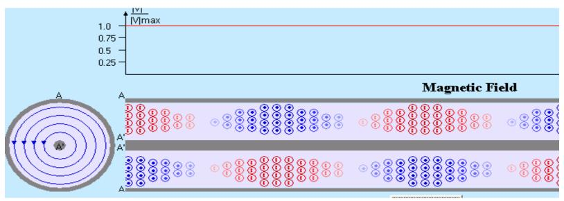
H-field in coaxial line. Orientation depends on phase - position along the line
