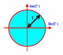
The domain of definition of the reflection coefficient is a circle of radius 1 in the complex plane. This is also the domain of the Smith chart.
