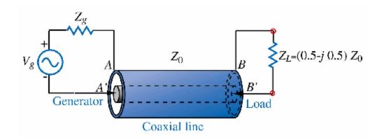
Coaxial line terminated by an impedance different than the characteristic impedance.
