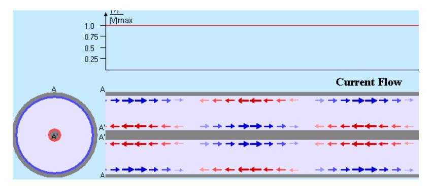
Surface current in coaxial line. Orientation depends on phase - position along the line.
