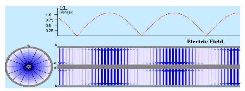
E-field in coaxial line. Orientation depends on phase - position along the line.
