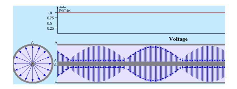
Voltage on coaxial line does not depend on time and position, because the load is matched.
