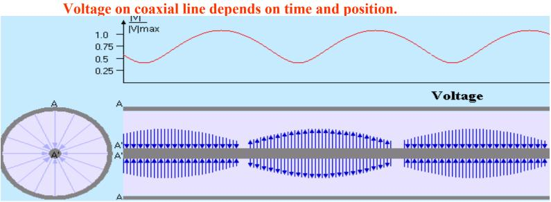
Voltage on coaxial line depends on time and position, but does not go to zero.
