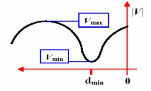
For a capacitive reactance, a voltage minimum is closest to the load and
