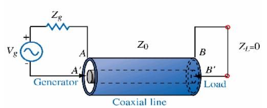
Coaxial line terminated by short circuit. The VSWR=indefinitely large.
