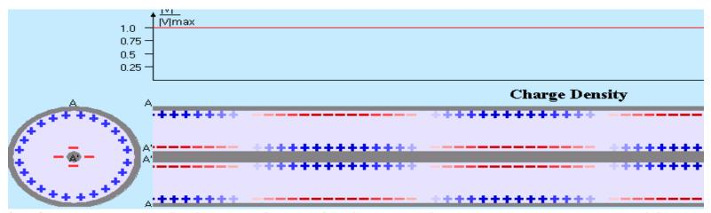
Surface charge density induced in coaxial line. The sign depends on phase - position along the line.
