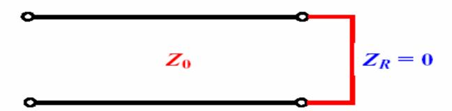
The load boundary condition due to the short circuit is V(0) = 0
