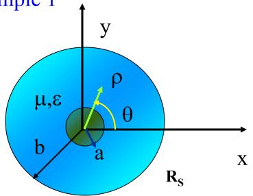
$$\overline{E} = \frac{V_0}{\rho \ln(b/a)} e^{-\gamma z} \hat{\rho}$$
