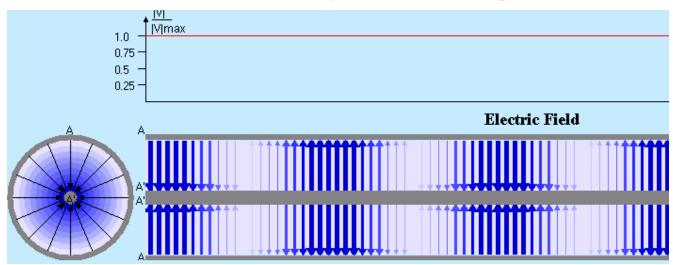
E-field in coaxial line. Orientation depends on phase - position along the line.
