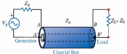
Coaxial line terminated by characteristic impedance.
