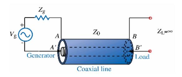
Coaxial line terminated by open circuit. The VSWR=indefinitely large.
