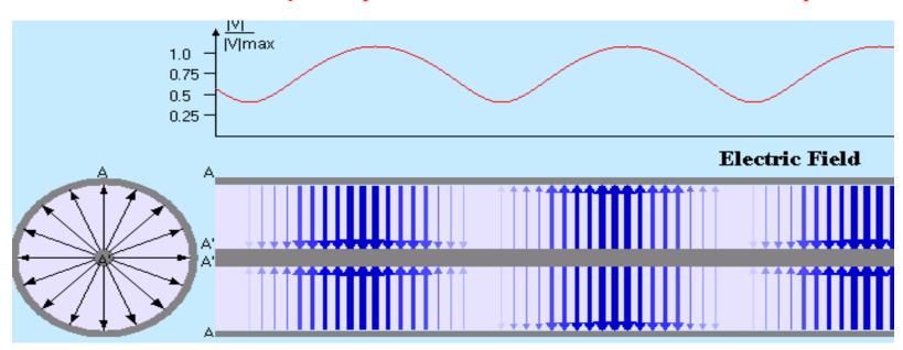
E-field in coaxial line. Orientation depends on phase - position along the line. The VSWR depends on reflection coefficient.
