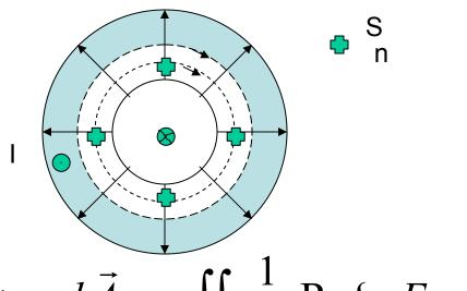
$$P = \iint_{S_{ab}} \langle S \rangle \cdot d\vec{A} = \iint_{S_{ab}} \frac{1}{2} \operatorname{Re} \{ E \times H^* \} \cdot d\vec{A}$$
