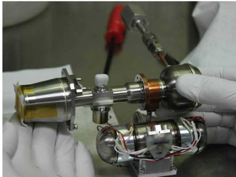
Figure 3. Integrated Dewar Detector Microcryocooler Assembly (IDDMA).
