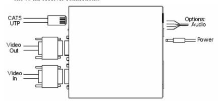
Figure 1: Transmitter Connections
