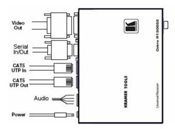
Figure 4: Cobra R1300S2 Universal Receiver Connections
