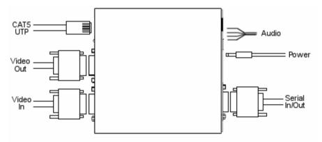
Figure 3: Transmitter Connections
