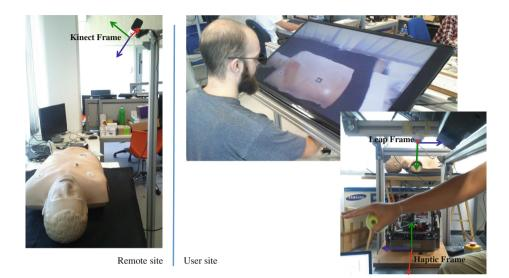
Fig. 3. The virtual palpation system. The hardware components are shown along with their reference frames.
