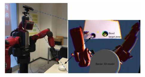
Fig. 5. The Baxter robot, on the left, with the Kinect mounted on the head. On the right the image displayed in the Oculus Rift
