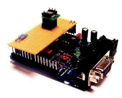
Accelerometer mounted on prototyping board, by M. Yarza
