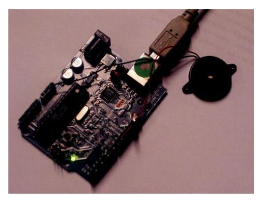
Example of connection of a Piezo to pin 9
