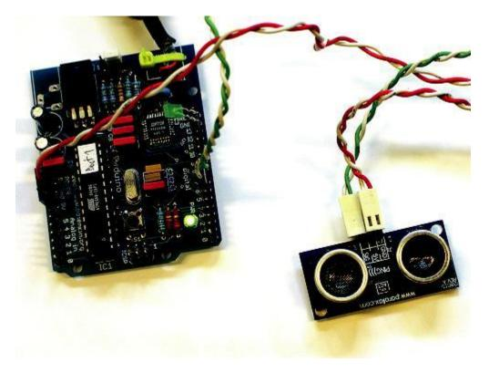
Ultrasound sensor connected to an Arduino USB v1.0
