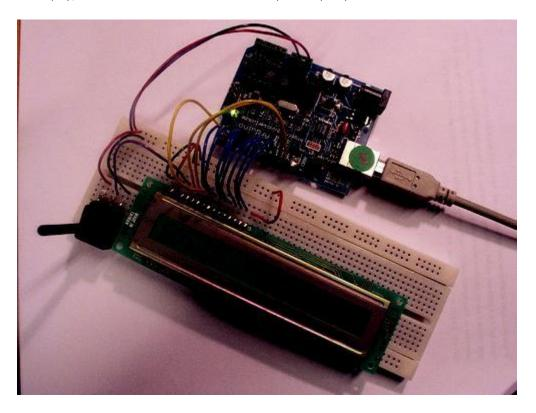
Picture of a protoboard supporting the display and a potentiometer
