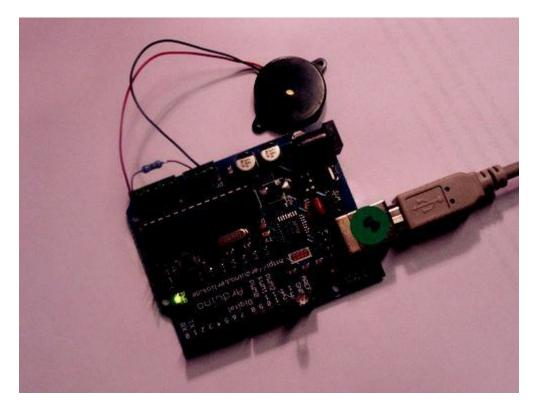
Example of connection of a Piezo to analog pin 0 with a resistor
