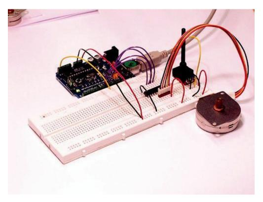
Picture of a protoboard supporting the ULN2003A and a potentiometer
