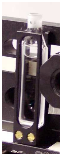
Fig. 20. Fused silica cell for the forward CARS (Starna Cells, 21-I-2).
